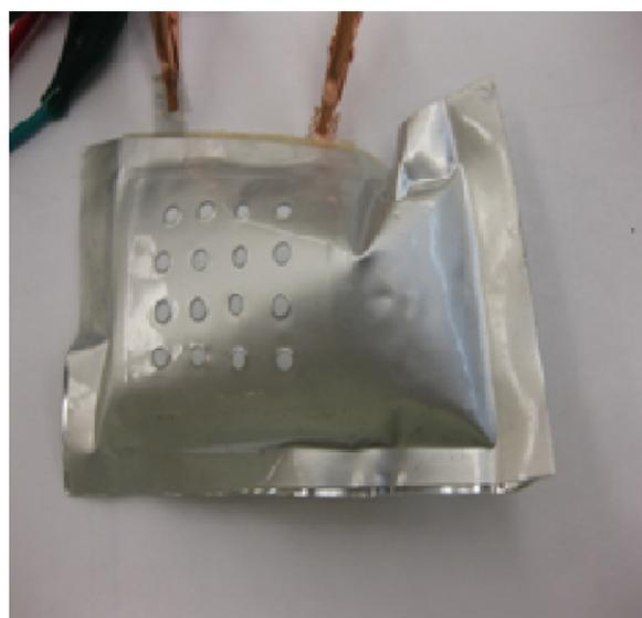
**Fig. 3.** Expansion of a G2 cell after discharge in ambient conditions.
